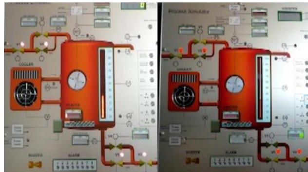
Figure 4. Digital Twin (l.) Simulated and Controlled by [6] with MATLAB ®/Simulink. The Hardware-model OSLO-3 (r.) Controlled with PLC Freelance and Field Controller AC-700 of ABB.
